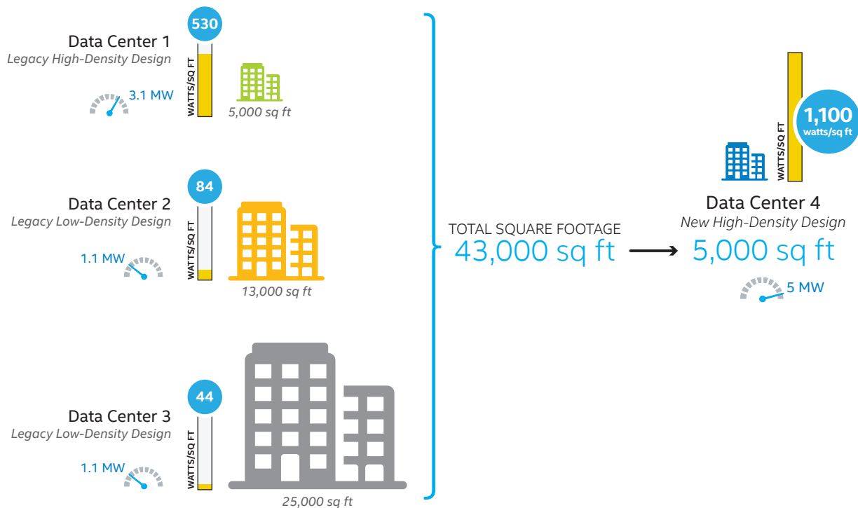
Figure 1. Our high-density design allows for an increase in watts per square foot. Economies of density work similar to Moore's Law: the cost per kW goes down as more kW are put into each square foot of production area.
