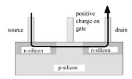
Although there are a variety of transistor types, all work in a similar way.
