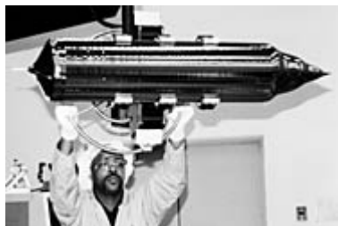
An ingot being prepared to be sliced into wafers (Photo: Ruth Carranzo Productions).
